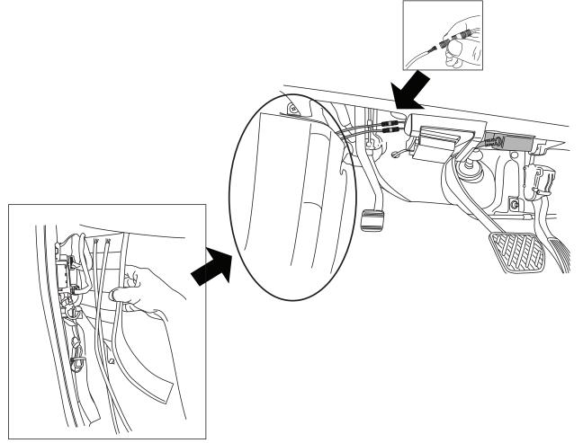
Use the Posi Locks(11) to make the connection to the plug and play module. Next plug in the Plug and Play(7) module under the dash as shown and route the wires behind the hood latch to the left. Make sure the wires are clear of the E-brake mechanism when it is on and off. The wires from below can be tucked under the carpet and covered with the trim reinstalled. Then reinstall the trim.
