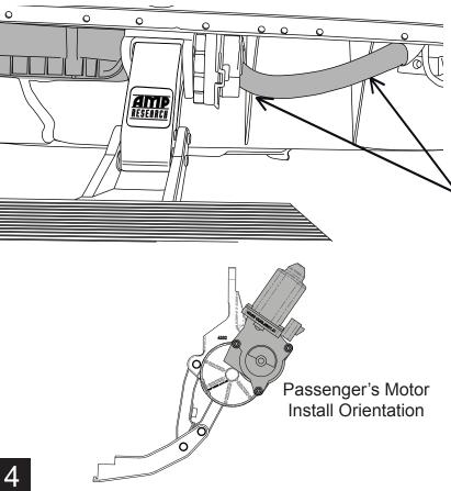
Assemble the motor to the linkage like the diagram below before installation. Position the motor so the linkage is in the most extended position.
