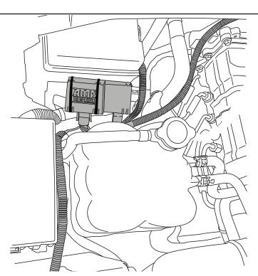
Next, connect the Black wire to the ground screw on the inner fender in diagram at top of page. Connect the Red wire to the stud on the positive power battery cable terminal.
