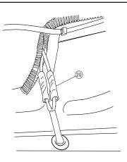
Using supplied butt connectors, connect the lamp wires. Red to Red, Black to Black. Once Crimped use heat gun to shrink tube.
