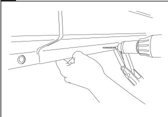
Center punch and drill a 1/8" pilot hole then drill a 19/64" hole through the pinch weld at marked locations. Deburr all holes. After drilling apply paint to holes to prevent rusting.
