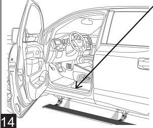
NOTE: Seal holes with silicone glue and cover with tape so carpet does not stick to glue.
