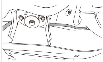
On the Driver side, Do Not Ziptire the Wire Harness to the Brake Lines.
