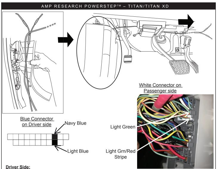
The short Trigger wire (purple with black stripe) needs to have a double diode crimped on as shown at left. Remove the connector block with 2 screws, the back side of it has a BLUE connector with both trigger wires in it. Connect one diode to the navy blue wire and one to the light blue wire (shown in diagram above) with Posi Taps(item 24). Re-install the connector block and trim piece, keeping the wire tucked away.
