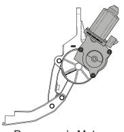
Passenger's Motor Install Orientation
