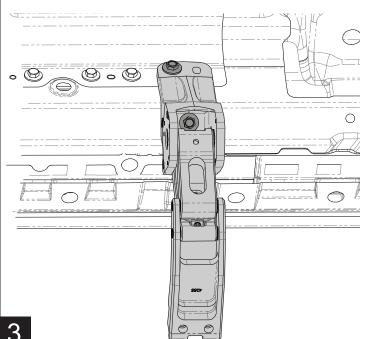
Next, install the Idler linkage in the **Third mount** position from the front of the truck. Install the upper bolt in the rearward hole. To install the lower bolt, put the bolt in a socket on an extension to guide it into position. Keep the linkage held up to the angled surface and vertical surfaces while tightening the bolts. **Torque fasteners to 16 ft-lbs. (22 N m).**
