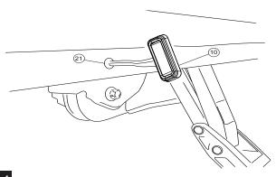
Insert grommet(21) into drilled holes. Insert lamp(10) wires through the grommets. (Silicon lube will help wires slip through grommets.)
