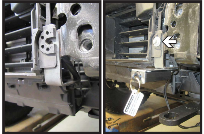
13. Optional Breakaway: Slide the breakaway bracket behind plastic piece and reinstall the existing bolt.
