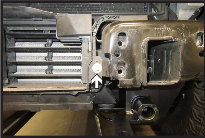
12. Optional Breakaway: Using a 8MM socket, remove the bolt from the driver side of the vehicle.
