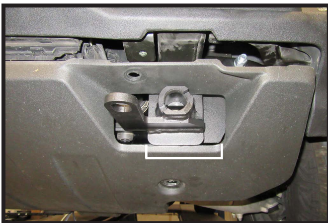
14. Hold the skid plate as close to its original position, mark and trim the skip plate around the convenience links and attachment tabs.
