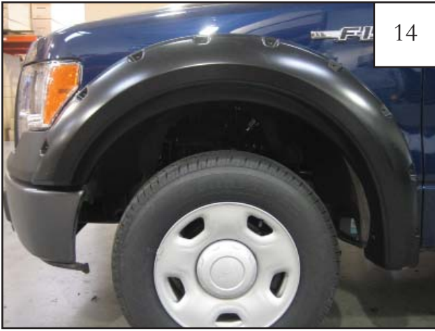
Completed front flare installation.
