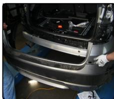
10. Remove (2) inner plastic bodies by removing (4) nuts from each.
