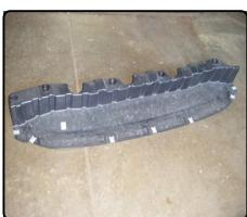
2. Remove (2) fasteners from bottom of bumper cover and (1) fastener from inside wheel well on each side. These are located behind rear tire. Some models may require removal of (1) plastic rivet from bottom of bumper on each side.
