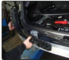
11. Remove bumper beam assembly by removing (4) nuts from threaded studs. These nuts will be used to install hitch.
