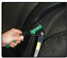
16. Raise underbody panel into position and mark the center using the hitch as a guide. Trim underbody panel. See UNDERBODY PANEL TRIM DIAGRAM on PAGE 2. Reinstall underbody panel and discard extra fastener. Install is complete.
