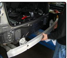
12. Raise hitch and bumper beam into position onto threaded studs and secure to vehicle using the M12 nuts removed in STEP 11.
