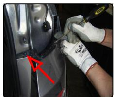
8. Pop (2) reflectors off of bumper cover and remove (1) fastener from under each.
