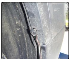
4. Remove (2) fasteners from each side of bumper cover which are now accessible due to wheel well trim removal.
