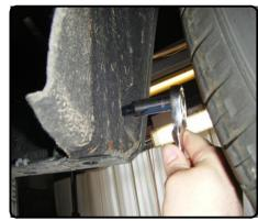
3. Remove (7) rivets from wheel well trim from above each rear tire. To remove rivets push small center rod though rivet with a small punch or an equivalent tool. Pry rivets from trim and pop trim off. **Note:** Replacement rivets are included.
