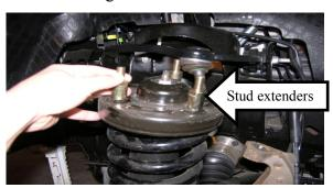
8. Install the spacer lift on top of the strut plate.
