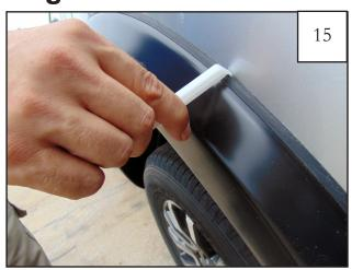
Using supplied Edge Trim Tool (Item 5), seat edge trim against vehicle by hooking curved end under edge trim at one end of flare. Next, slide around outer edge of flare to the other end.
