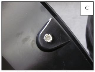
Place a Nut (Item 9) over the end of each Bolt and tighten, using a 1/2" wrench for the Nut and the supplied Torx Bit (Item 10) for the Bolt. Repeat for remaining pockets.
