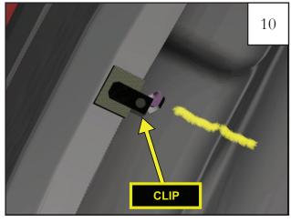
Install (6) (Item 1) long "U" clips on the center of the foam tabs.
