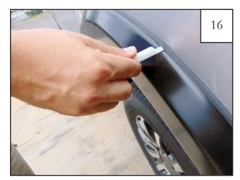
Using flat end of supplied Edge Trim Tool (Item 5), seat edge trim against flare by inserting straight end between edge trim and flare at one end. Next, slide around entire edge to the other end.
