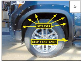
Install front flare using (6) (Item 2) truss screws and the (2) screws removed in Step 1.
