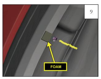
Install (6) (Item 3) foam tabs around the stock fender trim where the grease pencil marks were made.
