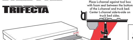
NOTE: These instructions are for adding a tonno to an existing truck tool box. They are supplemental to steps in the regular installation instructions included with your tonno.
