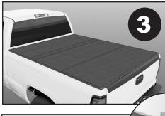
Unfold the cover all the way open to align cover on the truck bed rails before clamping.
