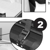
2. Undo both tie-down straps so cover can be unfolded.
