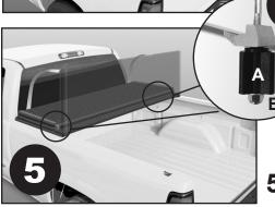
**4**. **A**. Tighten the plastic knob so that the hook is securely fastened to the metal bed rail.
