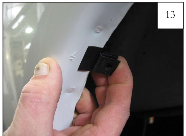
Slide a Clip (CL1-0005) over each Tab (MT1-0014).
