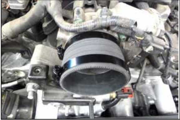
17. Install the hose with clamps to the throttle body and tighten clamp on throttle body only. Tighten clamps using 5/16" socket or nut driver.
