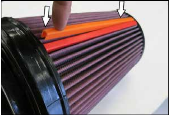
13. NOTE: Attach the filter clips to the pleats on the air filter align and push down. Driver side filters, place orange clip on top and red on bottom.
