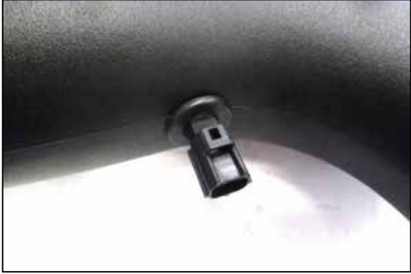
18. With provided grommet, attach to the hole on the intake tube. Install the temperature sensor into the grommet.
