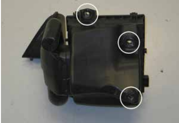
10. Remove three factory airbox mounting grommets from the lower airbox.
