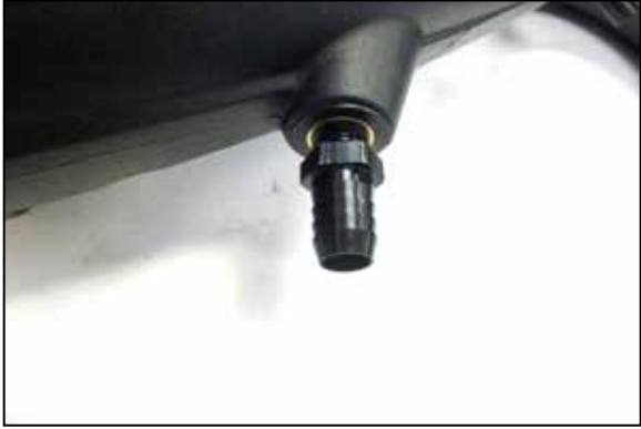
19. Install the provided barb fitting into the K&N intake tube.
