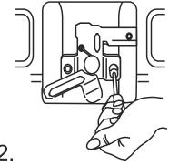
Unscrew the two nuts using a 10MM wrench holding the handle assembly. DO NOT CLOSE TAILGATE FROM THIS POINT ON.
