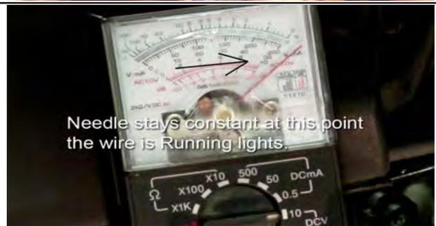
If the needle bounces on the meter, the wire is a turn signal. The voltage to the turn signal pulls high and low in order for the turn signal to blink. We don't recommend to
