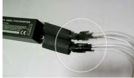
The CCFL wires comes with a heat shrink wrap, use a heat gun or a lighter to shrink the plugs together. When using a lighter, make sure to heat on the wrap and not on the wires itself.
