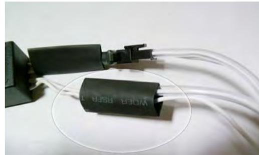
Connect the CCFL Inverter with the L.E.D. wires Using the quick connect, connect the CCFL inverter Positive(white). Same goes with Negative wires
